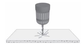
If screw joining into the Kerrock surface is required, a metal or PVC insert must be inserted. Observe work conditions which apply for glass or other more fragile materials. The borehole must be approx. 10% bigger than the screw's diameter. A rubber or silicone spacer must be used between the Kerrock surface and screw and the second material with screw joints.
