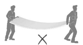
The sheets must be transported individually in a vertical position, where one hand serves as support and the other for control. It is recommended to use vacuum accessories for transporting heavy loads.
